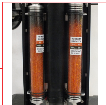
Silica gel desiccants in the fixture arm
