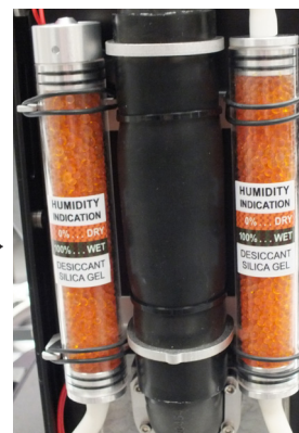
Silica gel desiccants in the fixture arm
